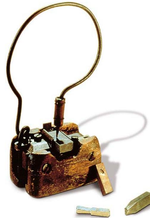
Hand casting instrument for casting lead type
